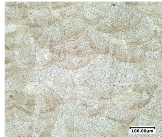
Microstructure of Invar36 after HIP
