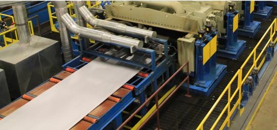
Samuel Nelson Technology, part of the family of Samuel companies, designs and builds complete process sections for hydrochloric acid (HCl) pickling lines for clients worldwide. Samuel Nelson Steel also owns and operates its own push-pull pickling and slitting line in Ontario, Canada to serve customers in the region.
