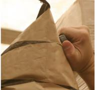
Remove inflator and attach valve cap. Ensure that cap is tightly secured.
