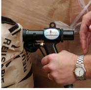
Squeeze trigger to begin inflation. When air blows out of the back of the inflator, desired pressure has been achieved.
