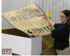
Place air bag into container. Weight of additional air bags will complete deflation process.
