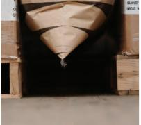
Position the air bag at least 1" above the floor to keep if from rubbing in transit.
