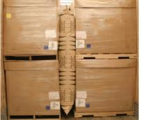
Create a bulkhead. The air bag is properly installed when Zebra stripes touch lading. If stripes show, and you can read the warning "if you can read this, the void is too large", deflate air bag and reduce the void.
