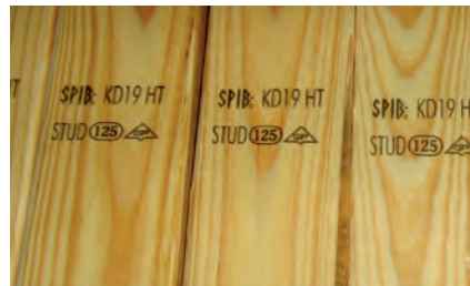
INK JET GRADE MARKING SYSTEM Proven non contact marking on lumber.
