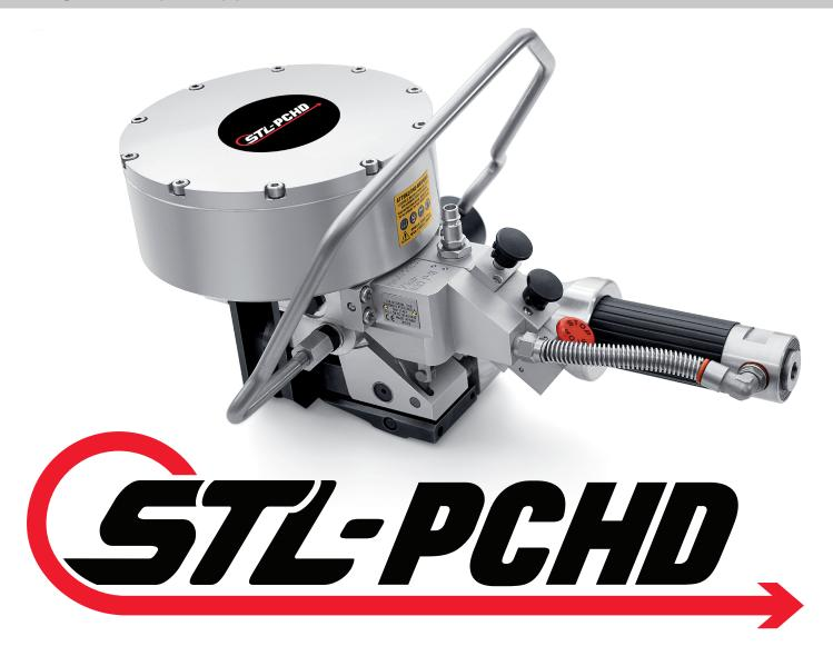
The STL-PCHD is a double notch upcut pneumatic combination tool that is used for high tensile round or irregular surface applications. It is a powerful and reliable strapping tool designed to be used in heavy duty industrial applications. The STL-PCHD uses push/closed seals to maximize seal strength. The STL-PCHD also includes a suspension bracket for standard and vertical applications.
